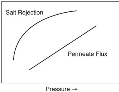
As shown in Figure 2, water flux across the membrane increases in direct relationship to increases in feedwater pressure. Increased feedwater pressure also results in increased salt rejection but, as Figure 2 demonstrates, the relationship is less direct than for water flux.
