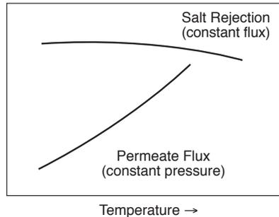
Increased feedwater temperature also results in lower salt rejection or higher salt passage. This is due to a higher diffusion rate for salt through the membrane.
